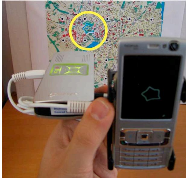
**Figure 1:** Prototype of a Map Torchlight unit in use. The castle of the City of Münster, Germany, is highlighted with a frame of white light (marked in the figure with a yellow circle). By clicking the center of the 4-way button on the phone the user can access detailed information about the castle history on the phone screen.
