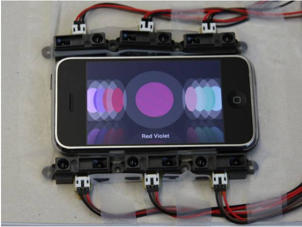
Figure 2. The current set-up of our prototype. Six Sharp GP2D120X IR distance sensors are placed along the long edges of an iPhone mobile device running the HoverFlow application (described in Section 3). Using simple hand gestures, the user can scroll and select colors in the color palette.
