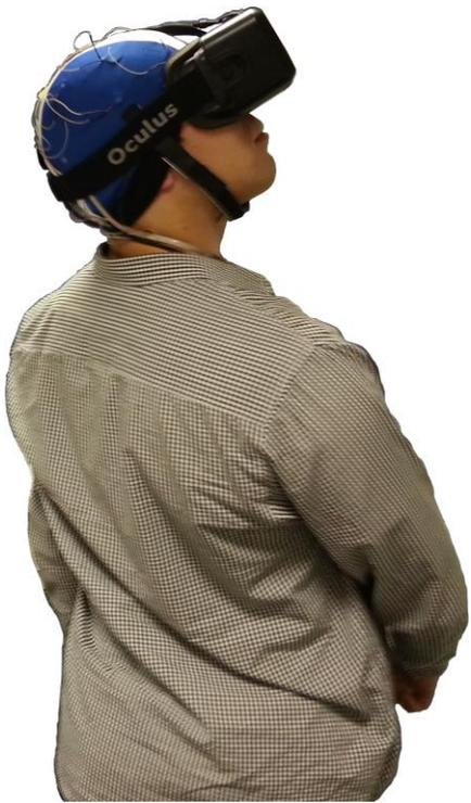
Figure 3: HapticHead prototype combined with an Oculus Rift for a tactile virtual-object-search-task.
