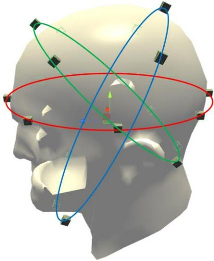
Figure 1: HapticHead concept modeled in Unity, side view. Note the three concentric ellipses around the user's head and no motor close to the ear's opening. The red ellipse contains 8 equidistant actuators, the green and blue ellipses each contain 6 actuators.
